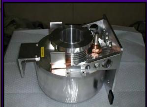
Accelerator target for Isolde, CERN, Genewa
